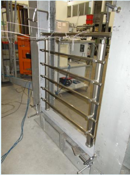
Photographs of the sample during resistance to horizontal static loading test
