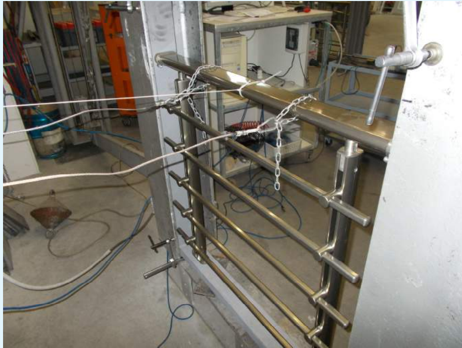
Photograph of the sample during resistance to horizontal static loading test
