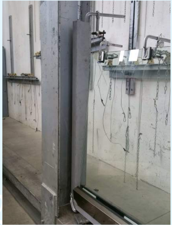
Photographs of the sample during resistance to horizontal static loading test
