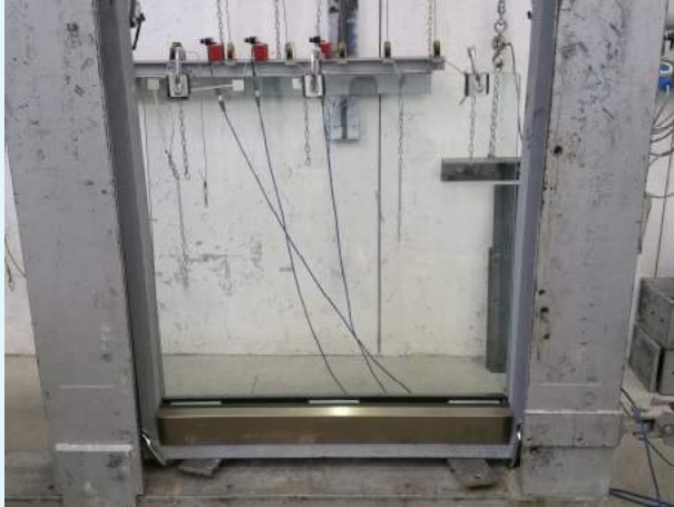
Photographs of the sample during resistance to horizontal static loading test
